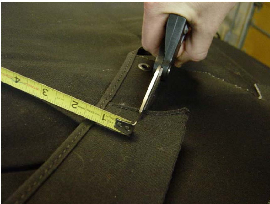
Figure 38: Trim the flaps that are glued into the rear quarter window channels.
