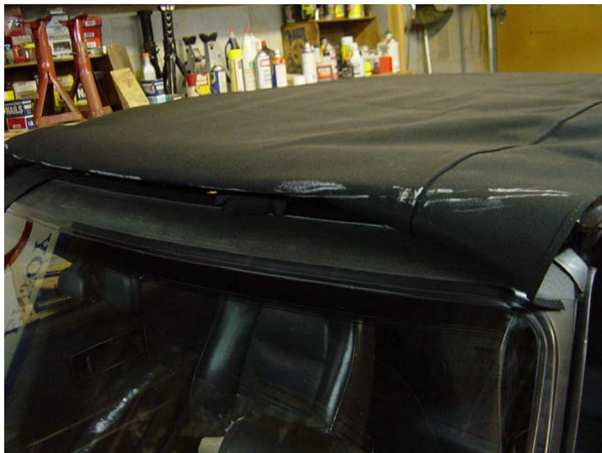
Figure 31: Checking fit with just middle of front bow glue dry.
