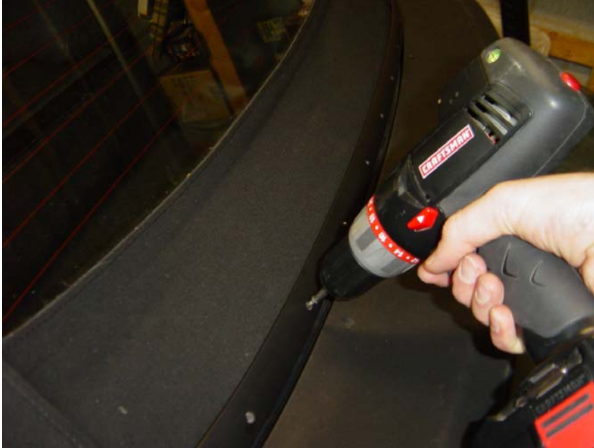
Figure 43: Installing rear trim strip over the staples.
