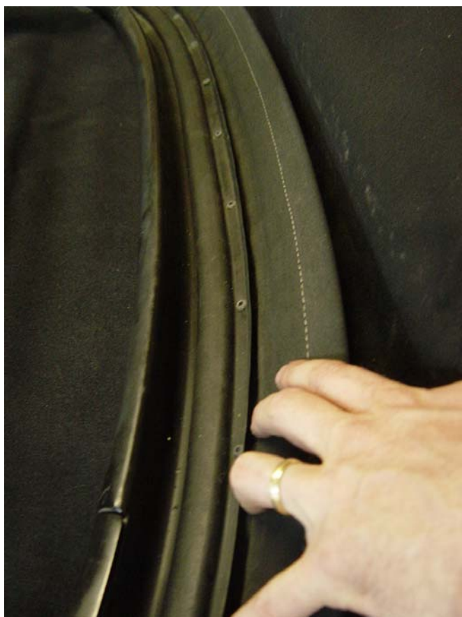
Figure 36: Wind stop secured, tucking under weather strip; ready to screw weather strip back down.
