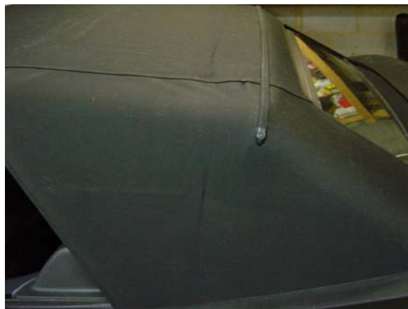
Figure 4: There is a little slack I was unable to eliminate in the seams near the corners of rear bow, but this is minor. If it bothers you, buy the German top.
