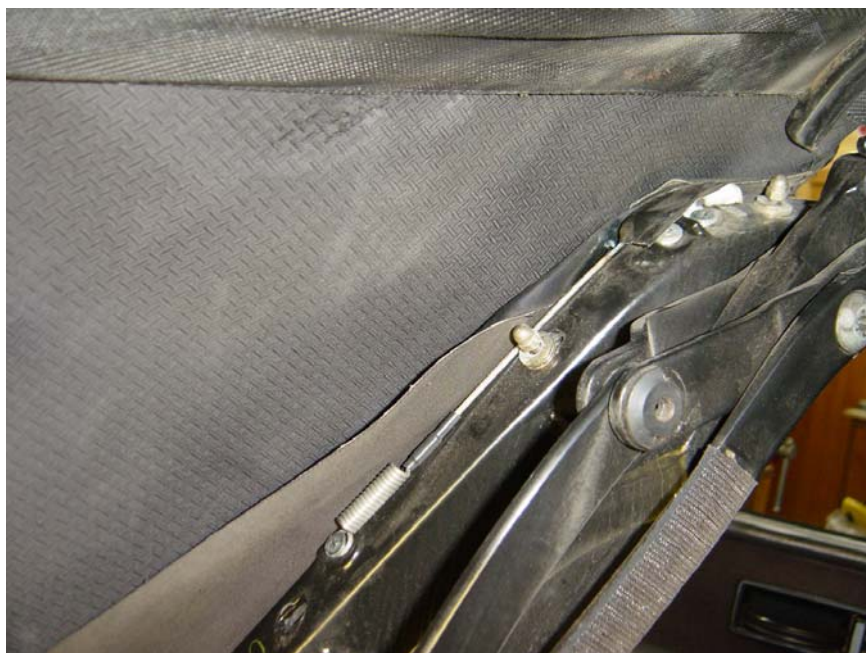
Figure 10: Removing weather strips from above the rear quarter windows. The holes above and below the coil spring are where torx screws were; I have not yet removed the two cap nuts toward the upper right of this photo.
