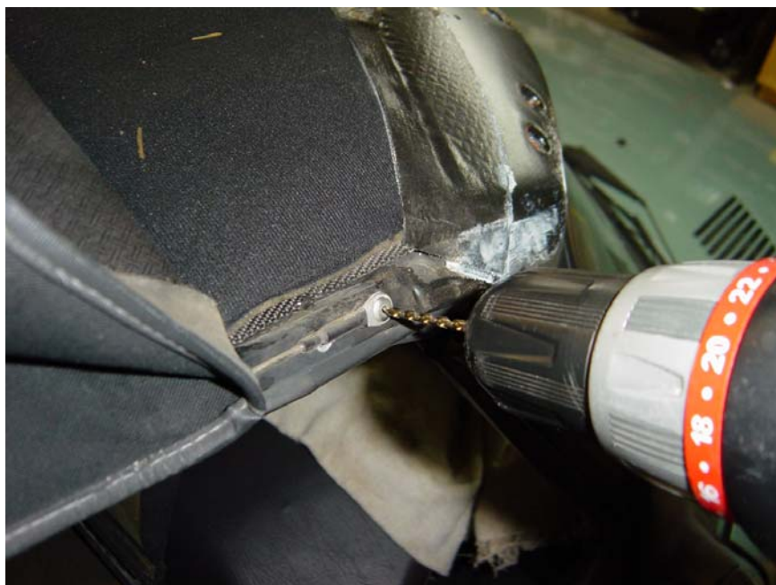
Figure 9: Drilling out pop rivets that hold the side cables at the front corners of the top. I started with 1/8" and finished with 9/64, then used a dental like tool to clean out the old rivet parts from back side of the hole. There is some black caulking that gets messy here – use adhesive remover to clean your hands and tools.
