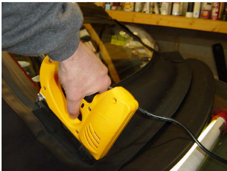
Figure 20: Stapling in bottom of rear window section. Keep the extra fabric (to right of staple gun in this photo) until you absolutely must trim it in case you mess up.
