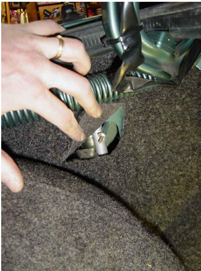
Figure 12: Accessing wing nut in trunk that holds down the rear of the side spoiler.
