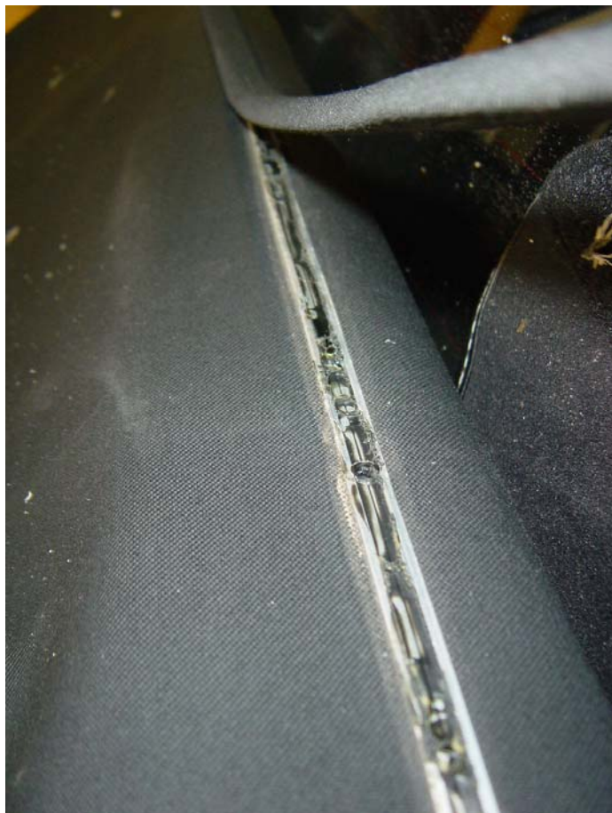
Figure 13: Removing trim strip across the top of the rear bow. Be careful because this will be reused.
