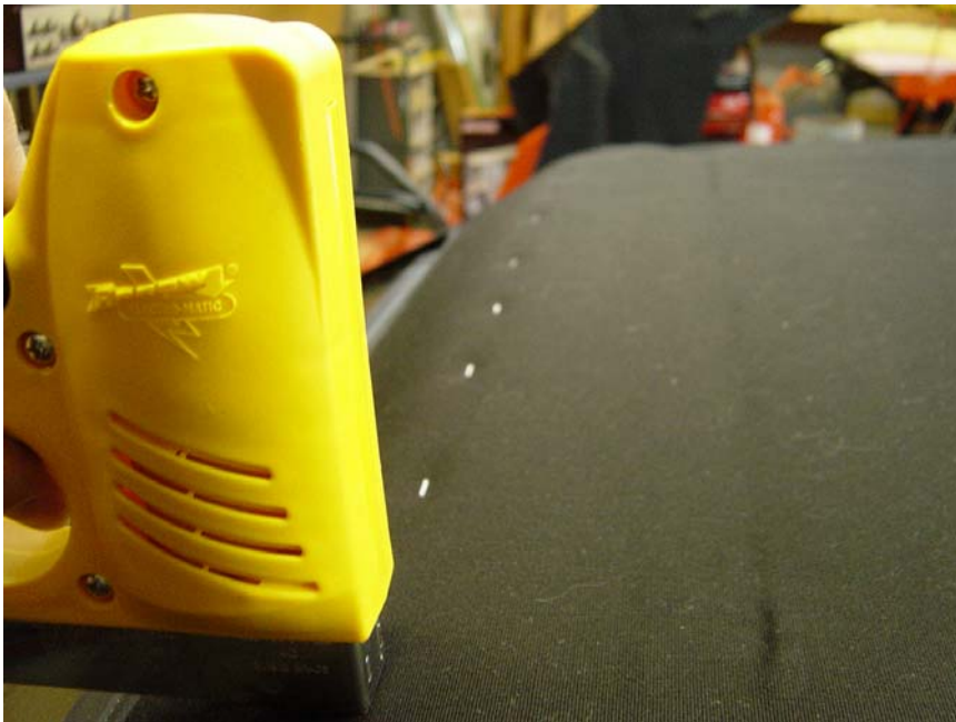
Figure 46: Stapling top to rear bow. It is critical the staples be in a straight line here so they will be hidden under the trim.
