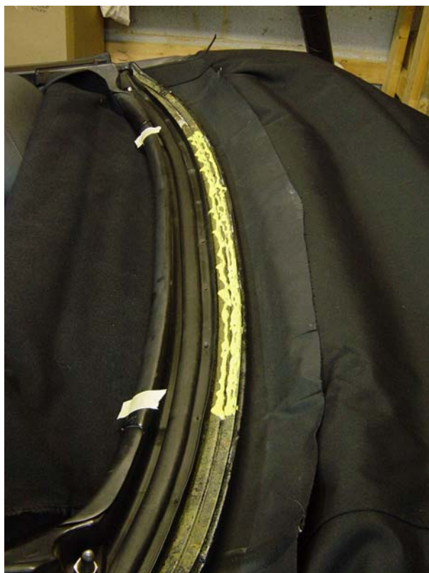
Figure 30: I glued the middle first (between the two spots of making tape) , let that dry, then checked the fit before I glued the outsides. Use lots of glue on the front bow because the staples do not hold well.
