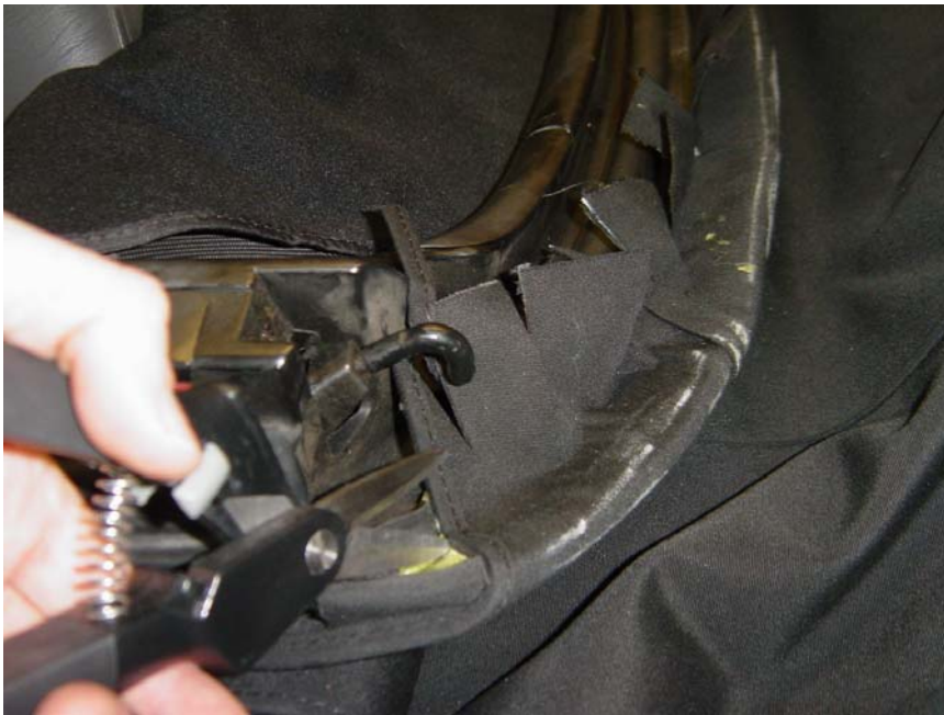
Figure 34: Cutting away excess fabric under front bow. Note the style of scissors (OXO with Off Ramp from Lowes) — these were perfect for this job.
