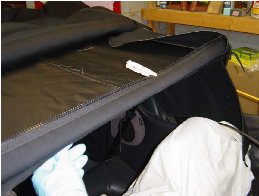
Figure 26: Securing headliner to rear bow. Note drop cloth to protect rear seat from gorilla snot and glove to protect my hand.
