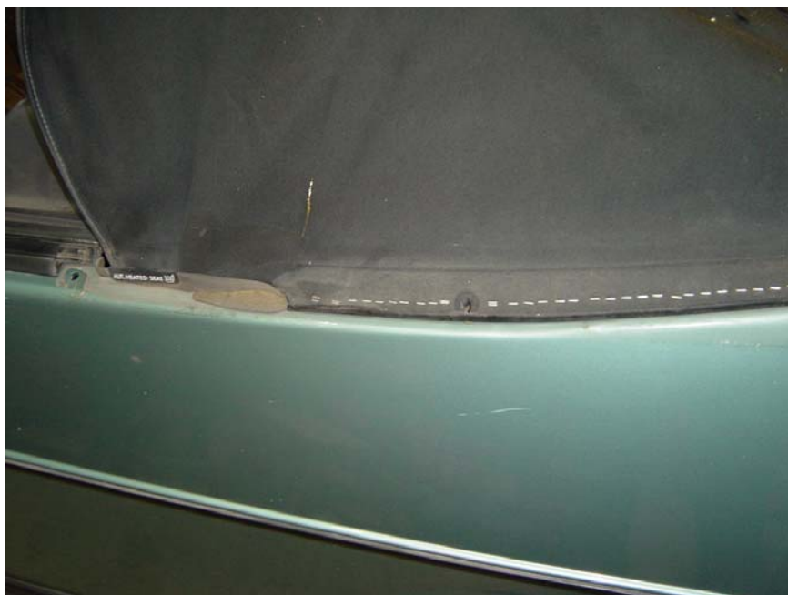
Figure 14: Side spoiler removed, ready to remove the top from the sides. Notice the large number of staples.
