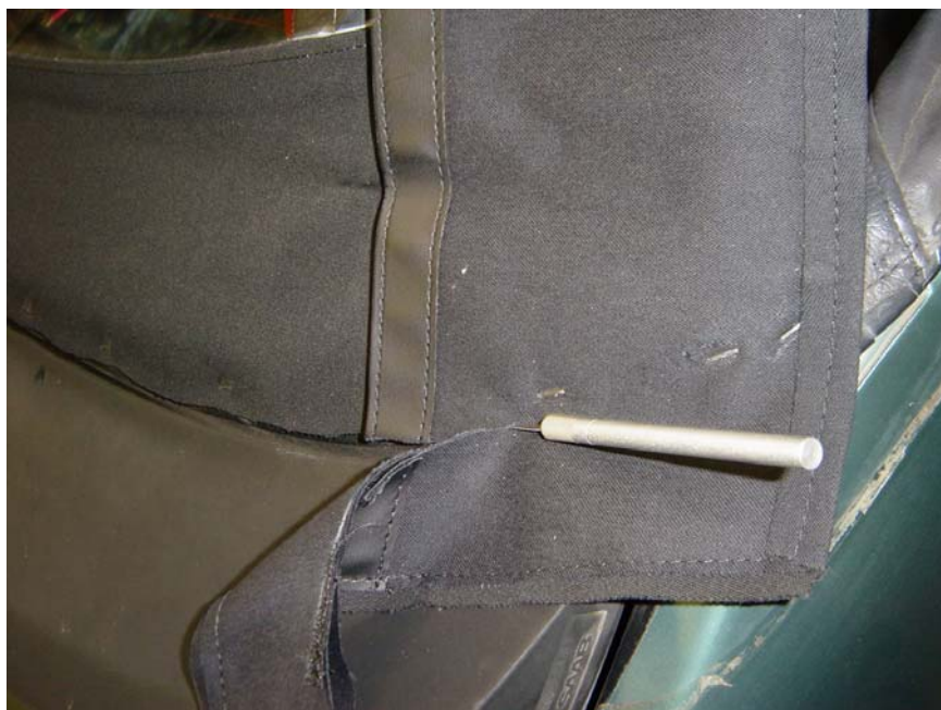
Figure 21: Here is my mistake that caused the gloss black vinyl to be shows at the top of the window (see After photos) -- I cut away the excess fabric before it was absolutely required. Also later I found the scissors shown in Figure 34 were a better tool for cutting than the xacto knife shown here.
