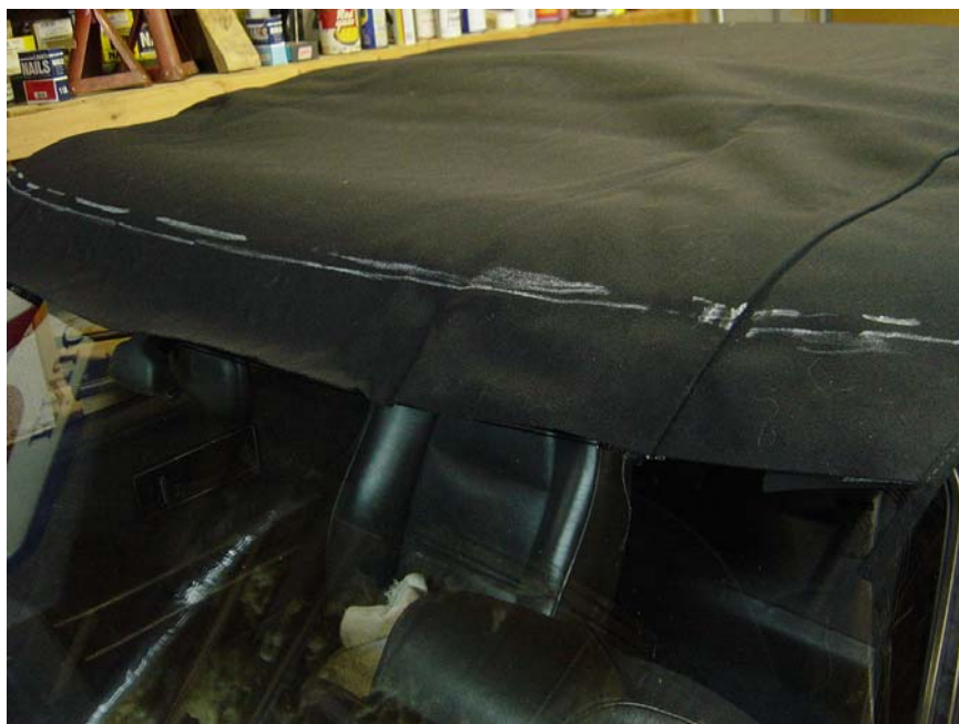
Figure 29: Soap marks across fabric at front bow to identify how to glue under front bow when top opened for gluing. I have three marks because it took me three marking efforts before it was right. You need a helper for this marking step.
