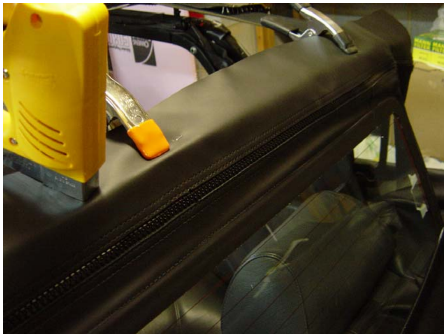
Figure 19: Stapling in rear window section.
