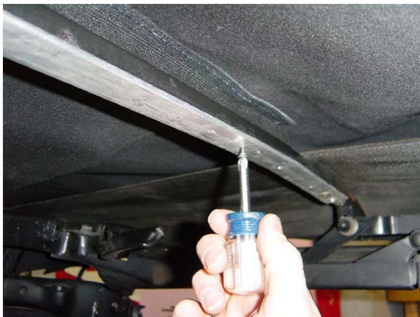
Figure 22: With top centered, install the retaining strips for the 2nd and 3rd bows.
