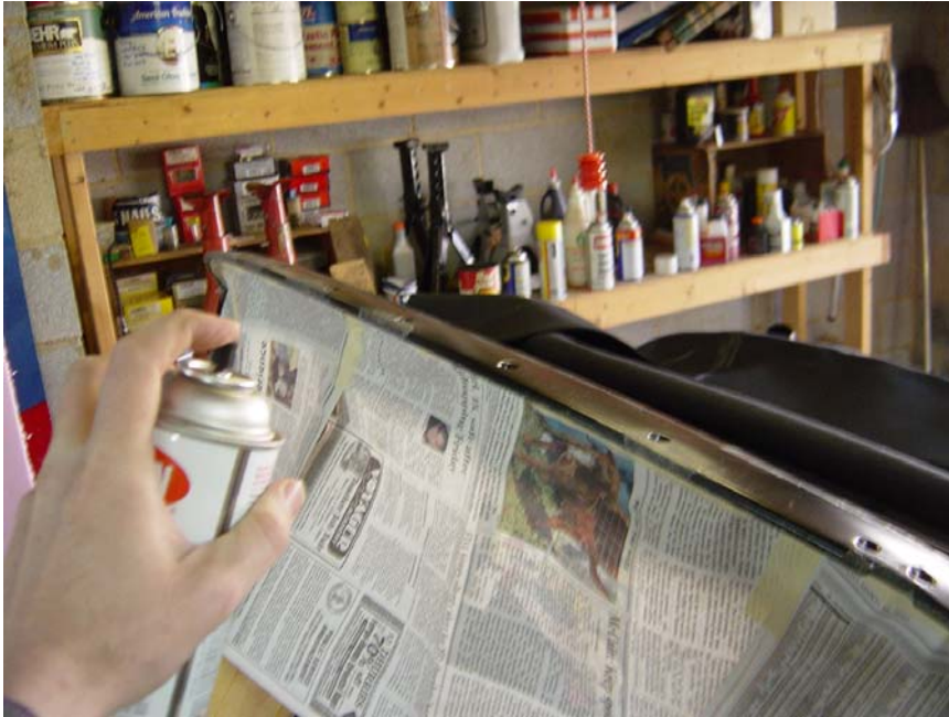
Figure 23: Painting to mitigate corrosion of aluminum front bow.
