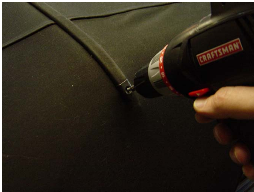
Figure 47: Last step of trim installation. I wanted to reuse the screw holes in the bow from the prior installation, but found that too difficult to locate. Installing the screws in new locations seemed to work pretty well.
