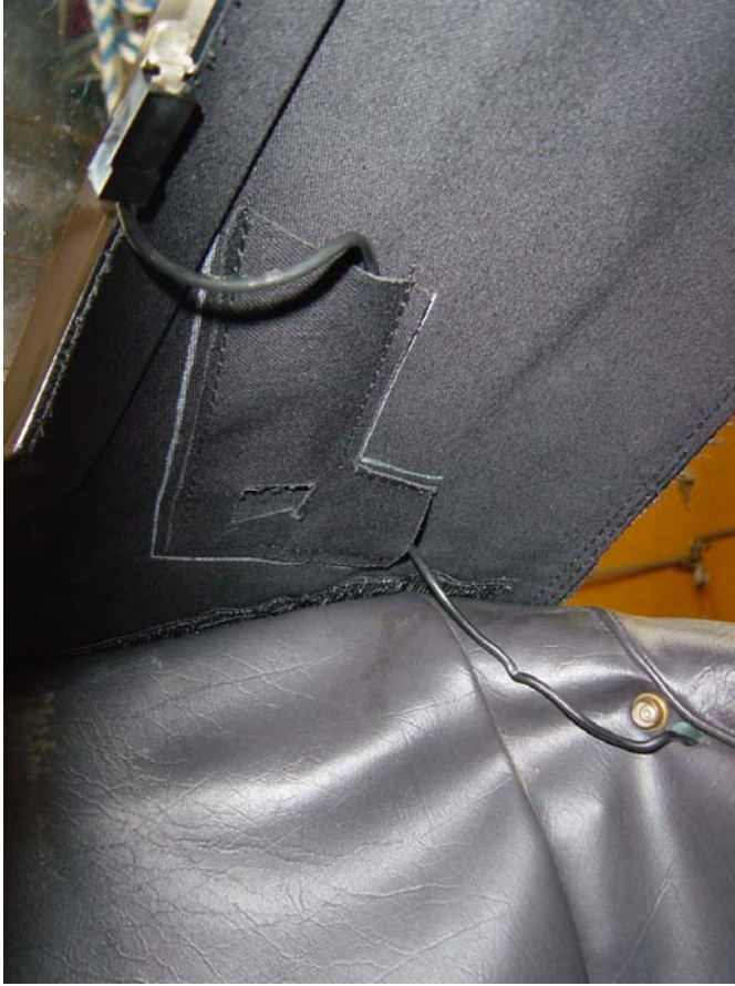
Figure 37: Snake the defroster wire thru the fabric. Note the Velcro for the headliner is partially hidden under the stapled area. This is another indicator I had the rear window section too low, but at this point I had already trimmed the excess fabric so I added self adhesive Velcro above the original Velcro.
