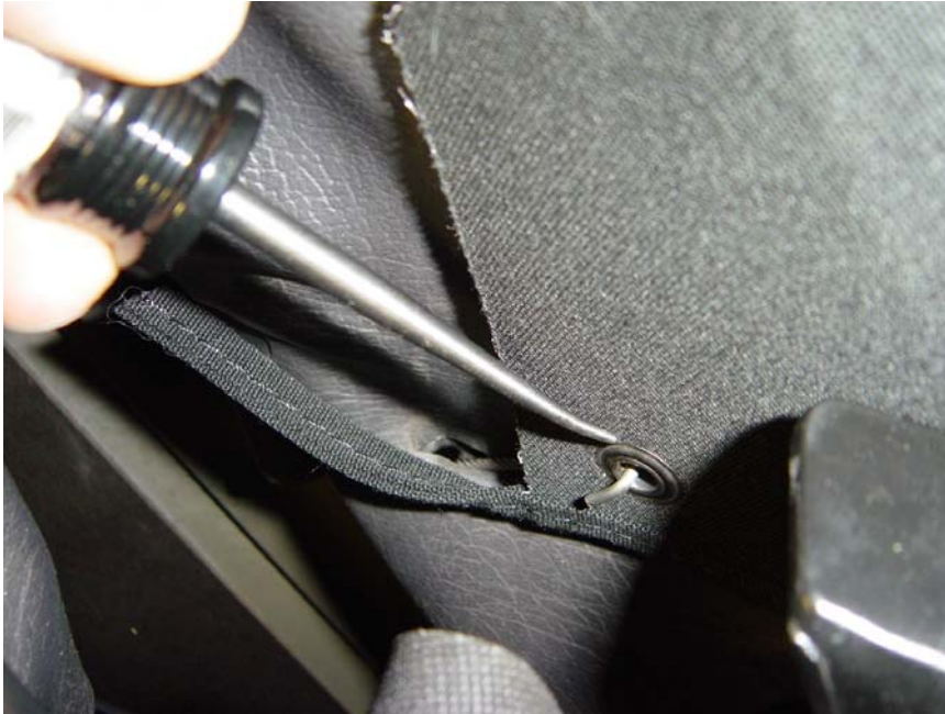
Figure 39: Attach springs at corners behind the rear windows.
