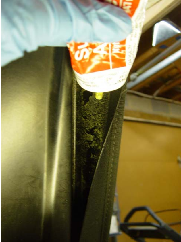
Figure 45: Gluing top to quarter window area.
