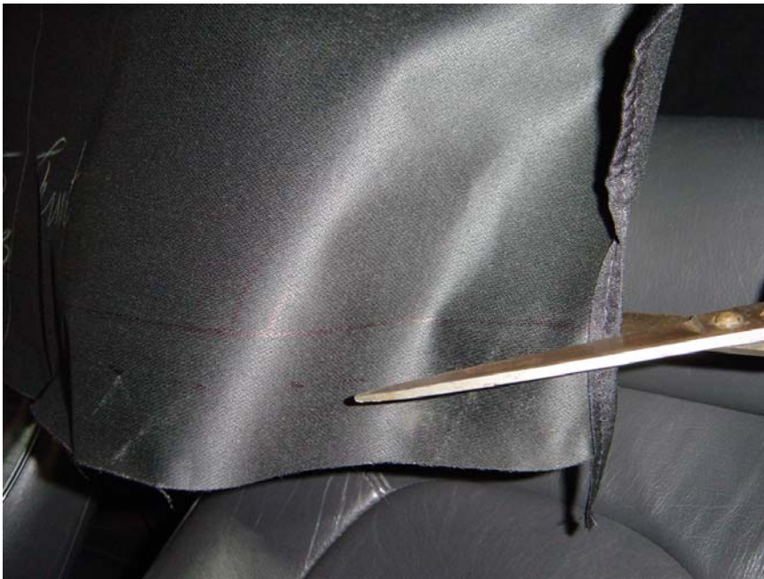
Figure 24: Trimming front of headliner. This must be fairly precise because no excess can protrude beyond the retaining strip at the first bow.
