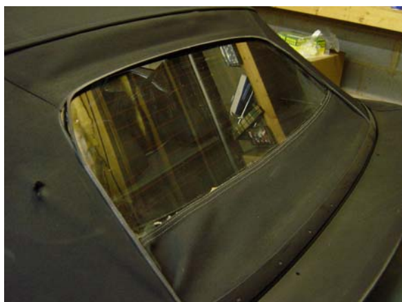
Figure 2: Rear glass separated from old top plus another hole on side
