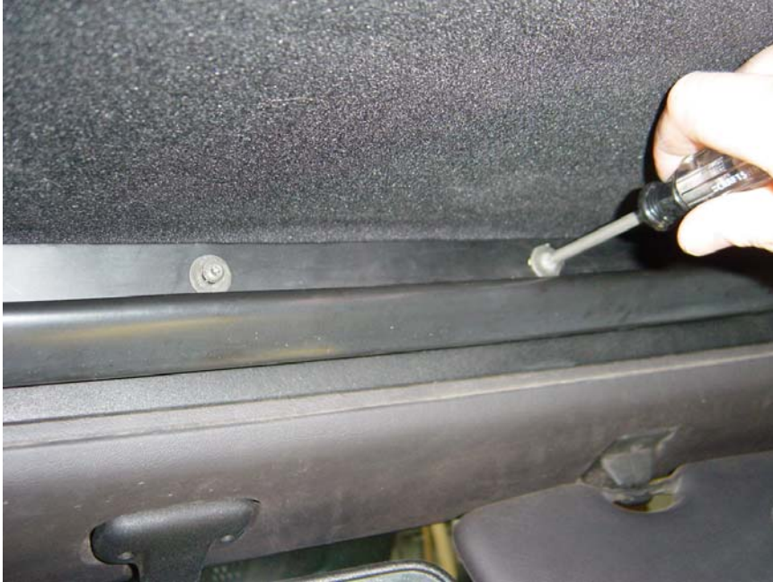
Figure 25: Installing headliner retaining strip onto front bow. It also has gorilla snot on its back side.
