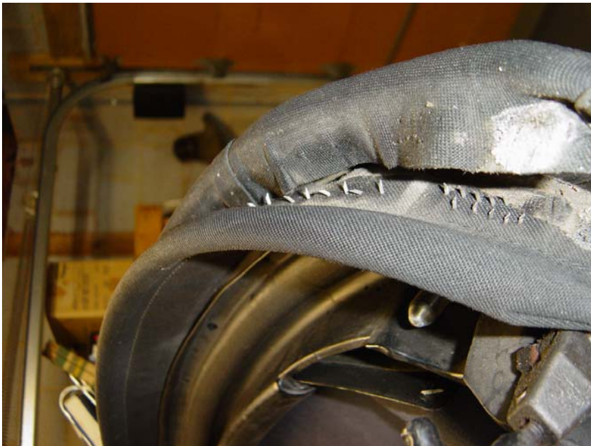
Figure 8: Removing wind stop and main top from front bow
