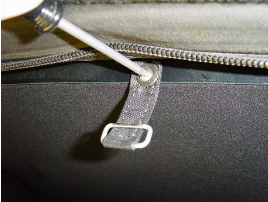
Figure 7: Removing fasteners connecting headliner to rear bow (not required unless replacing headliner)
