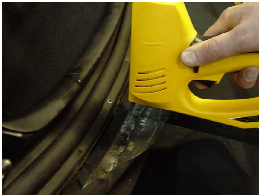
Figure 35: Stapling wind stop under front bow (staples go under the flap). These staples do not hold well so use adequate glue.
