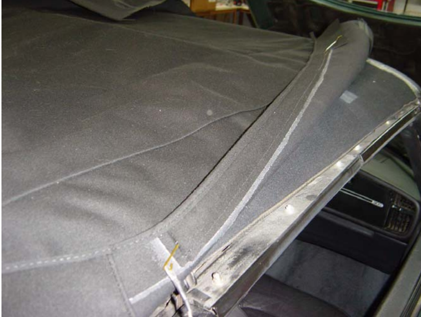
Figure 27: Using coat hangar to pull side cable into sleeve.
