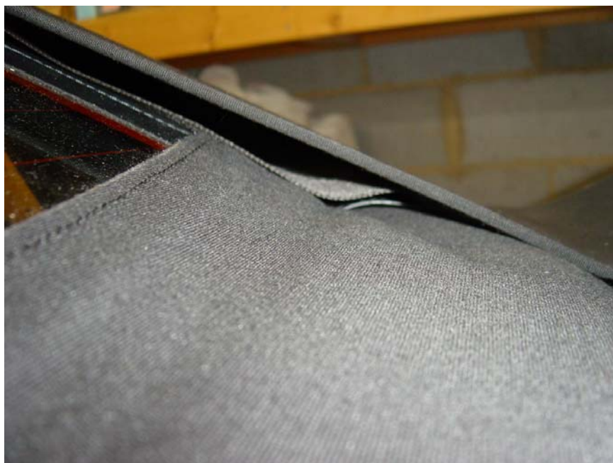
Figure 41: Here is a problem -- the tension of the new top when closed caused the rear window and the support strap above it to be loose. You can't know whether this will happen to you, just anticipate the top fitting will take extra time. I disassembled the rear section to retension the rear window and support strap.
