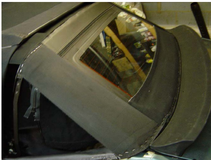
Figure 42: Here I have folded the top forward to access and retension the rear top assembly.
