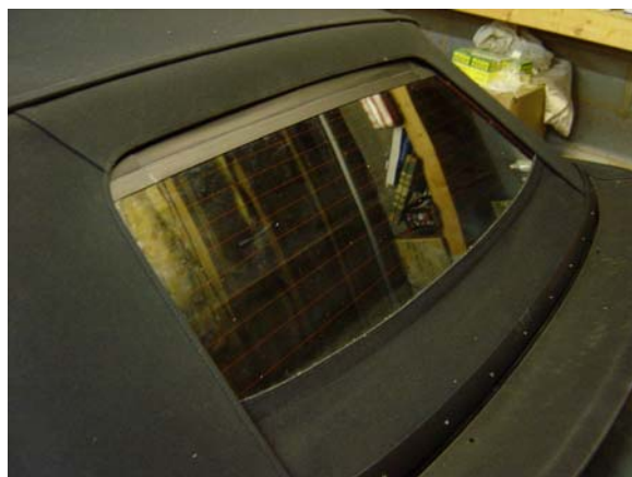
Figure 5: My window ended up being mounted a bit too low — my fault. The gloss vinyl above the window should really be hidden below the top fabric, but this is minor.
