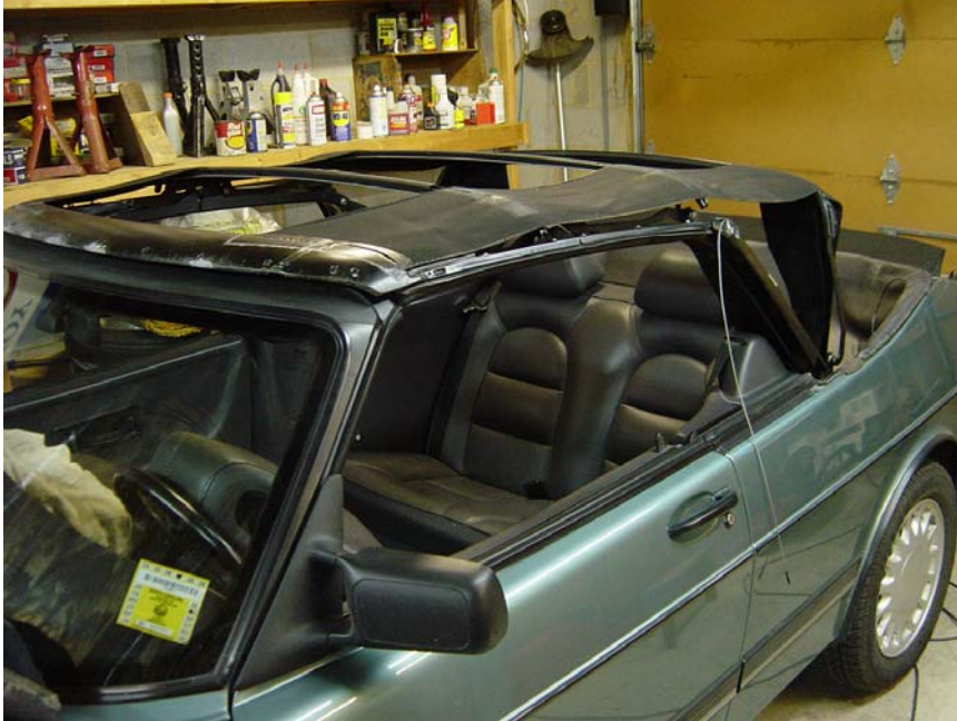
Figure 17: Top, rear glass section, and headliner now removed.
