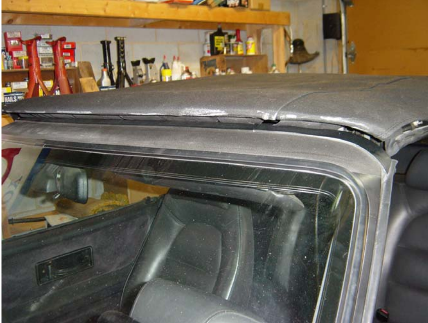
Figure 33: Now the whole length is glued, checking fit again before cutting away excess fabric.
