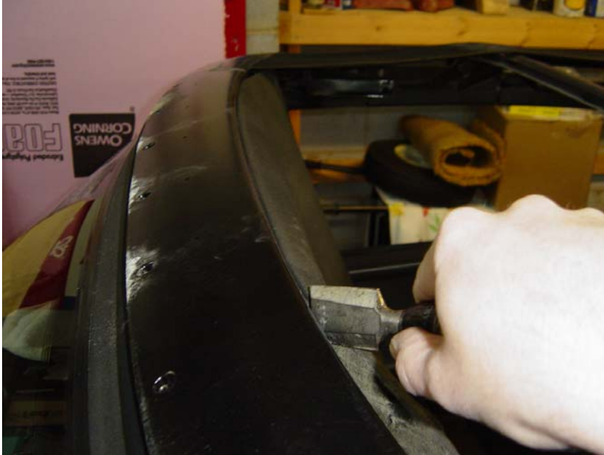
Figure 11: Removing the headliner from the front bow.
