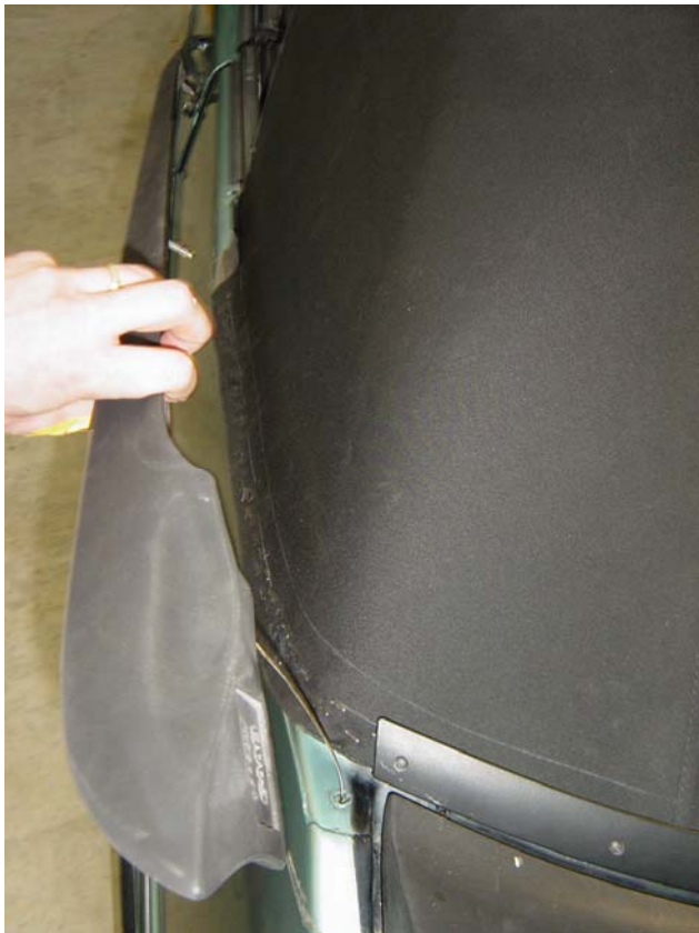
Figure 44: Installing side spoiler section. I was lucky, in my vehicle the middle threaded stud was simply that -- no nut to locate deep inside the body.
