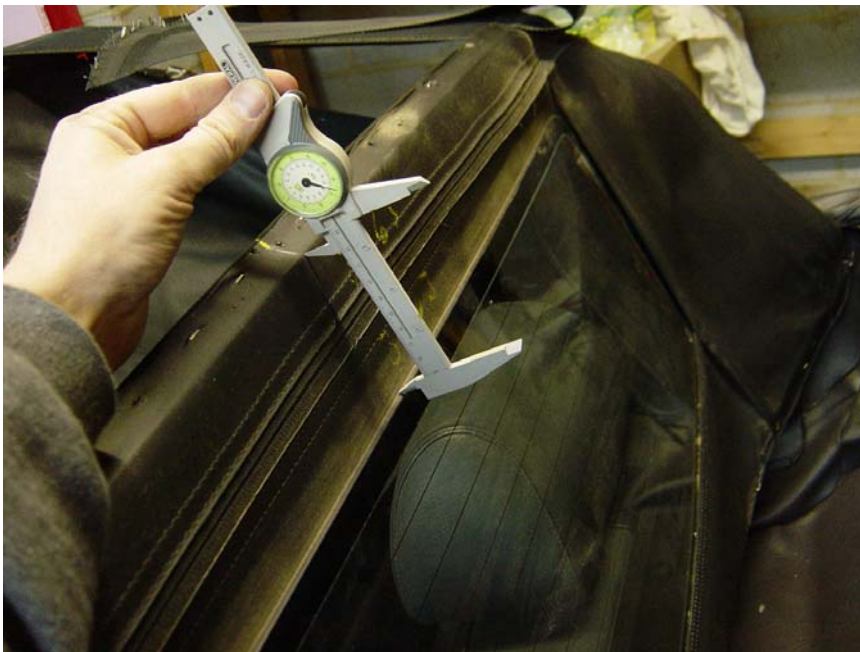
Figure 16: Measuring old glass section to be sure new glass is installed in proper position. Note the support strap (upper right of photo) that goes between the glass section and the main top.
