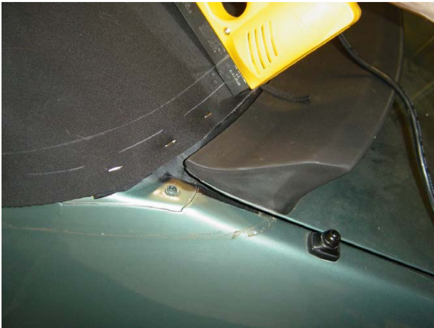
Figure 40: Stapling new top on rear. Note using a few staples now to check fit.
