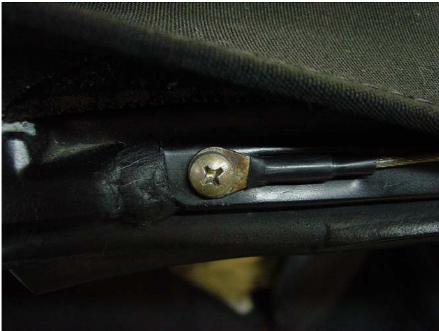
Figure 28: Sheet metal screw that replaced pop rivet for side cable.
